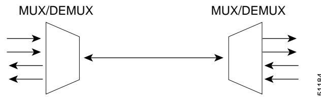
Figure 2-19 Multiplexing and Demultiplexing in a Bidirectional System
